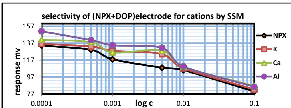
Figure 7: Selectivity of (NPX-MIP+DOP) electrodes with ions via Separation Solution Method.
