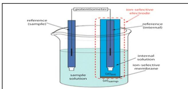
**Figure 4:** Schematic Diagram Showing a Typical Potentiometric Cell with an Ion-Selective Electrode.
