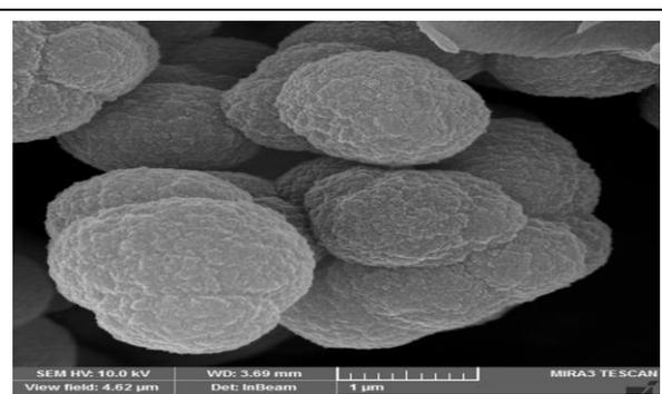
Figure 3: SEM for the MIP after washing
