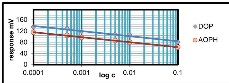
Figure 5: Calibration Curve for NPX-MIP Membrane Electrodes.
