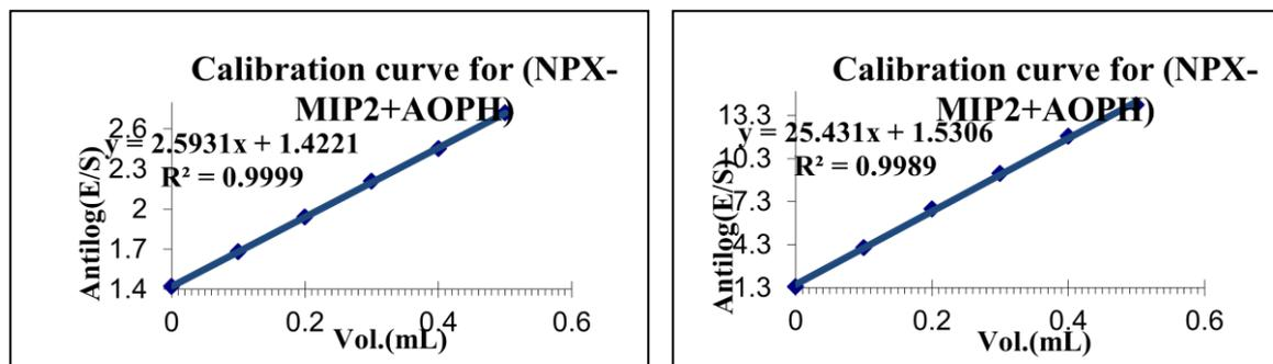
**Figure 10:** Antilog (E / S) against the volume of the added standard for the determination of Naproxen solution ( $5 \times 10^{-3}$  and  $5 \times 10^{-4}$ ) M by MSA using (NPX-MIP+ AOPH) electrode.
