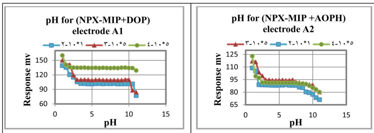
Figure 6: Effect of pH on the Naproxen {NPX -MIP+ DOP (A1) and NPX-MIP +AOPH (A2)} Electrodes at Concentration  $10^{-2}$ ,  $5 \times 10^{-3}$  and  $5 \times 10^{-4}$ .
