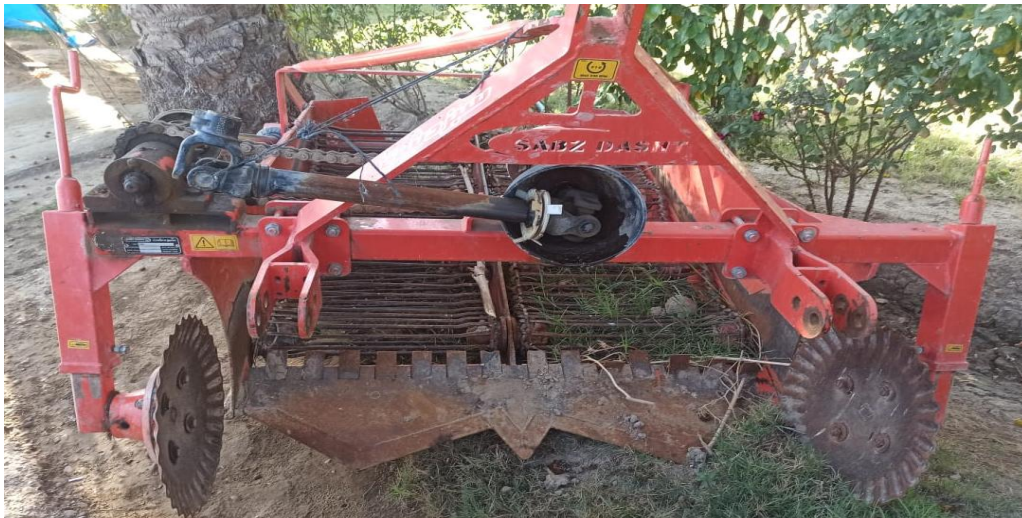
Figure (1): shows a front section of a potato digger
