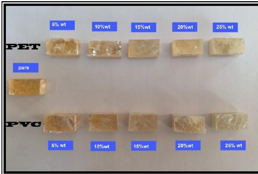
Fig. 3: Compression test specimens.
