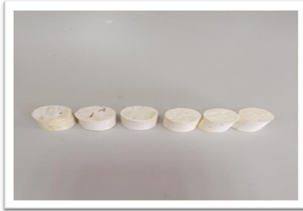
Figure (2): The shape of the sample prepared for compressive resistance testing.
